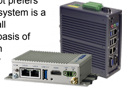
Fig. 7: DR2100 from TL-Electronic (background) and UNO-2271G from Advantech.
